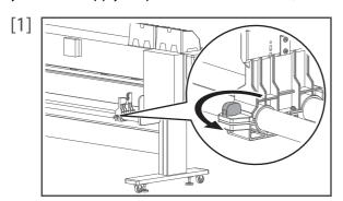
Twist the knob bolt on the right side of the media holder anticlockwise to loosen.
