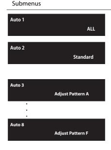
Perform automatic adjustment for all patterns (A to F) using the color sensor.
