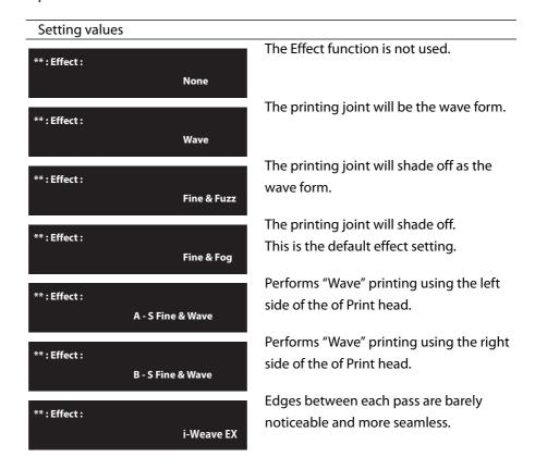
Type \*\*: 2 Adjust Print Sets up when adjusting the printer for the optimum quality of image print. Before adjusting this setting, enter the thickness of the media.
