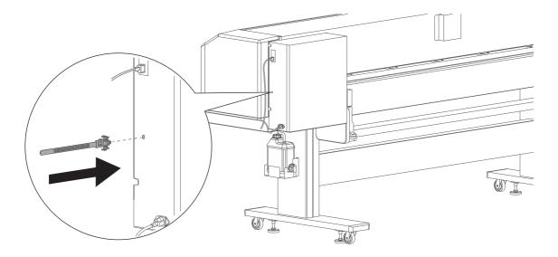
[3] Use the cable tie to secure the Ethernet cable to the printer.
