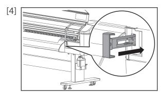
(To cancel the individual pressure rollers) Push the media feed lever back to the original position to lock the pressure rollers.
