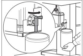
Open the waste ink valve and drain waste ink into the container.
