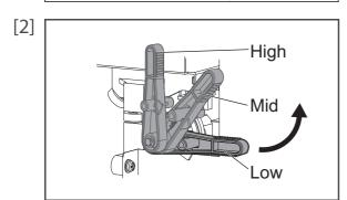
Use the head height adjustment lever (orange) to change the head height to "Mid" or "High".
