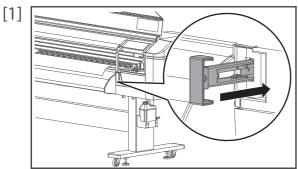
From the front side of the printer, push the media feed lever to hold the media flat with pressure rollers.
