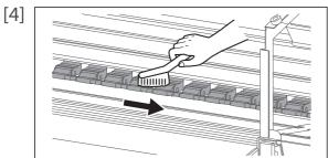
Brush off dusts on the pressure rollers with a soft brush.
