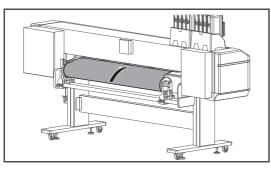
From the rear side of the printer, insert the front edge of the media into the media slot.
