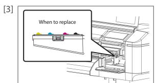
Check the absorption material for the flushing box.
