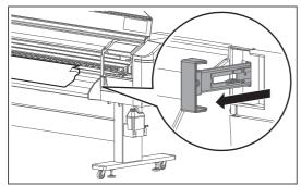
From the front side of the printer, pull the media feed lever towards you to release the pressure rollers.
