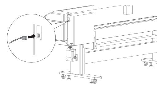
Insert the tip of the cable tie into the hole on the printer to attach it. [2]
