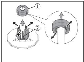
(If you are using 2-inch core roll media) Remove the 3-inch adapter from the media flange.
