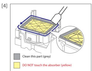
Use the cleaning stick to clean around the rubber part of the capping unit to remove the ink deposits and dust.
