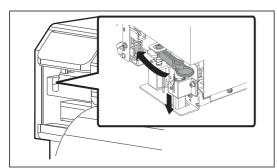
Press the cutter cap lightly, turn Cutter holder in the direction as illustrated below.
