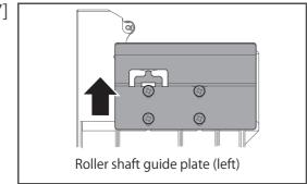
Do the same for the left media holder to slide up the roller shaft guide plate as far as it will go and tighten the screws.
