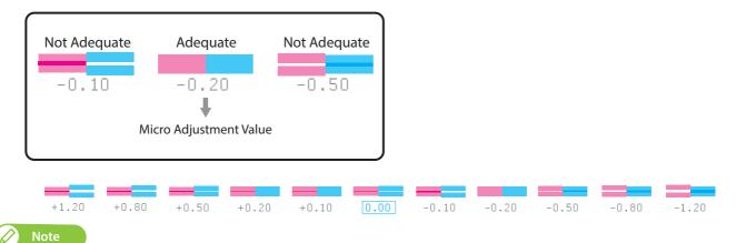
Once an appropriate micro adjustment value has been saved, the value will be the baseline value from the next time to be printed in the center of the pattern.
