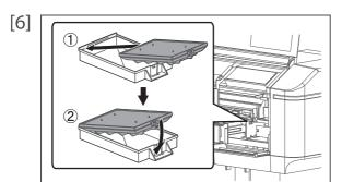
Attach new absorption material for the flushing box.
