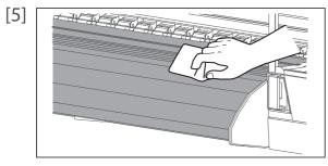
Use a soft cloth or paper towel slightly dampened with ethanol to clean off the ink on the platen, media guide and edge holder.
