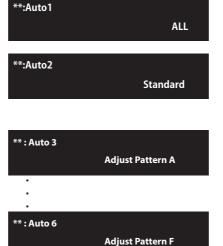
Perform automatic adjustment for all patterns (A to F) using the color sensor.
