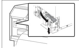
Press the cutter cap lightly, return Cutter holder to its initial position.
