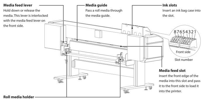
Attach the media flanges to both ends of a roll media and load it onto the roll media holder.
