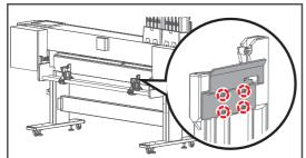
(When looking from the rear side of the printer) Use the screwdriver to loosen four screws securing the roller shaft guide plate to the right media holder.
